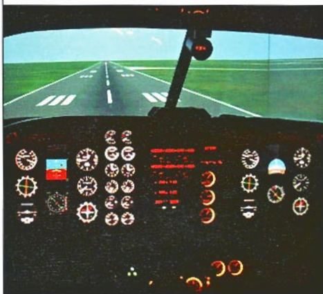
Mechtronix-built Ascent flight and navigation procedures trainer (FNPT II).
